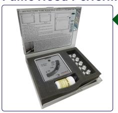
The Performance Test Kit measures face velocity and air flow visualization per ASHRAE 110-1995 procedure. Kit includes: vaneometer, 10 smoke candles, 20 smoke matches, test report manual and instructions. Can test up to 5 fume hoods.
